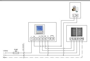
Intelligent PSH panel controls actuators/valves and automatically regulates fans' speed depending on the required room temperature. Fans speed changs automatically for lower rate, when temperature in a room gets closer to desired one.
