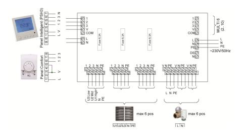
MULTI 6 Splitter allows to connect and control more fan heaters (up to 6 pcs.) and valves with actuators (up to 6 pcs.). Control of fans and valves is done using COMFORT or INTELLIGENT panel.
