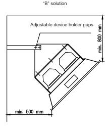
10. picture: Installation of the GH heaters and safety distances
