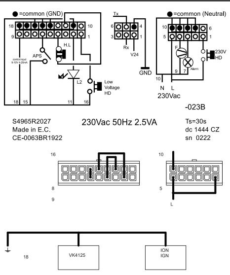
7. picture: Connection points of S4965R2027 automatic burner control
