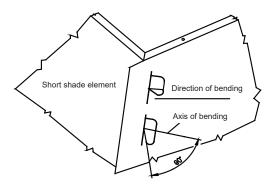
3.picture: Assemblage of the reflector
