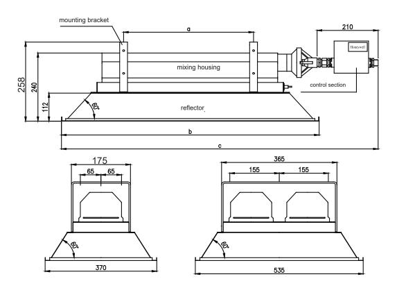
2.picture: Gas working infrared heaters types
