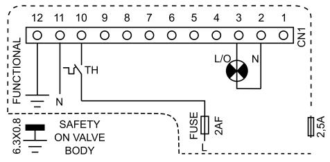
8. picture: Connection points of SIT 579 DBC automatic burner control
