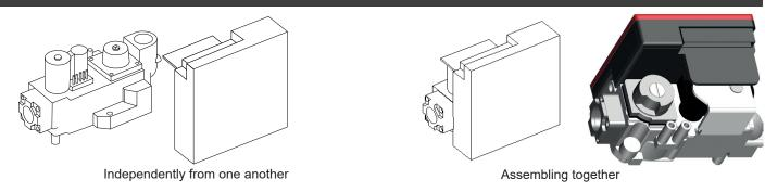
6.picture: Assemblage of the gas magnetic valve
