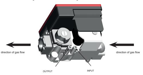
14. picture: Input and output gas pressure cheking connections in case of HONEYWELL solenoid valve
